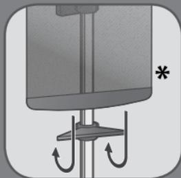
**EN** Unwind the support and insert it in the adjustable hook, by adjusting the tension with the dedicated hook and lock it.
