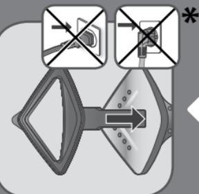
**EN** The crease attachment is used to make pant creases easily or to remove stubborn wrinkles. Put your fabric in the space between the two accessory parts. Move the crease attachment in a downwards motion starting from the top.
