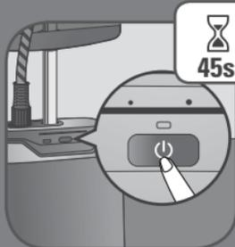
**EN** Push the ON/OFF button, in order to switch on the appliance. The leds will flash for approx 45 seconds.
