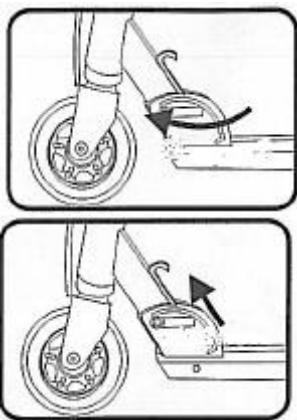
3. Open the locking mechanism.
