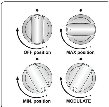
After ignition, visually check the flames. If you see a yellow tip, lifted or unstable flame, switch the gas flow off, then check the assembly of burner caps and crowns once they have cooled. Make sure there is no liquid in the burner caps. If the burner flames go out accidentally, switch the burners off, ventilate the kitchen with fresh air and wait at least 90 seconds before attempting re-ignition.
