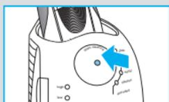
If the station selects one of the required cleaning programs, it will not start unless you press the «start cleaning» button ④. **For best shaving results, we recommend cleaning after each shave.**
